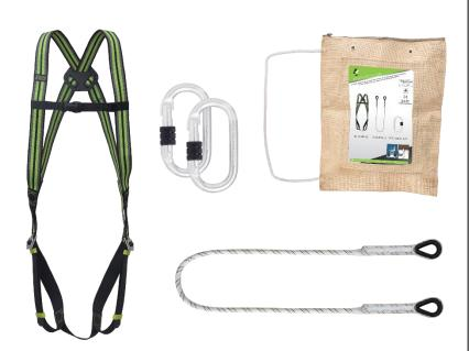
Minimalist, but complete, this set must be used where there is no risk of a fall, in restraint at work (prevents from accessing to the area of risk of fall).
